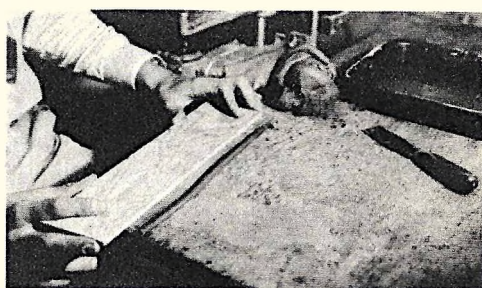
Suitable clay for pottery work may be secured from a local brickyard for a few cents. The clay is handled in the same manner as dough after which it is rolled out, as illustrated above, into long rolls using a flat board for the working tool. In making the coils it is advisable not to have the clay too moist, otherwise it may stick to the forming tools.
