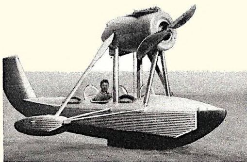
Speed boating reaches a new peak in thrills in one of these wingless seaplanes. A standard airplane motor and propeller lift the aluminum hull almost clear of the water at high speed.
