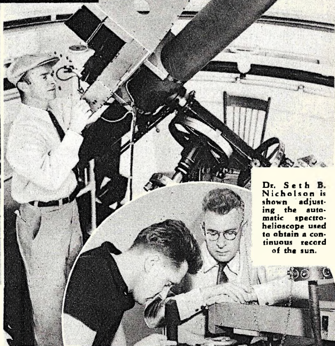
Circle — Here is Dr. Hickox experimenting with the filter device developed by Dr. Edison Pettit for measuring the sun's output of ultra-violet light.
