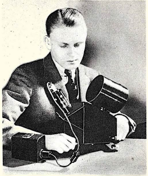
George W. Jacobus is shown here with his vibrometer, or vibration photographer. As a pool of mercury in its base quivers in response to vibrations, its movements are photographed from light rays reflected from a mirror on its surface.
