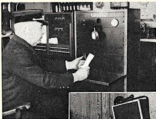
Chief Thomas Burns, of the Bridgeport, Conn., Fire Department broadcasts the first message over the Talkalarm, a radio fire alarm system. Inset shows loud speaker installed at fire station.
