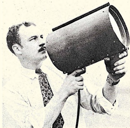
Pointing like a rifle and having triggers, this portable light throws colored beams for signaling purposes at Logan Field, Baltimore, Md. It replaces the old flagging system.
