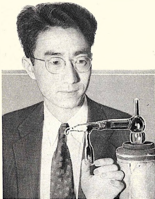
Chao-Ying Meng, Chinese research fellow of the Rockefeller Foundation is shown with the world's smallest radio tube which he built. It generates the world's shortest wave length.
