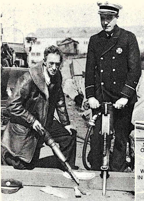
Supt. N. T. Woods, left, and Capt. Grenfell try out the pneumatic wood cutter and concrete driller, two tools necessary in boring through docks and floors. Once the hole is made, the special fire nozzle invented by Wood quickly quenches the fire.
