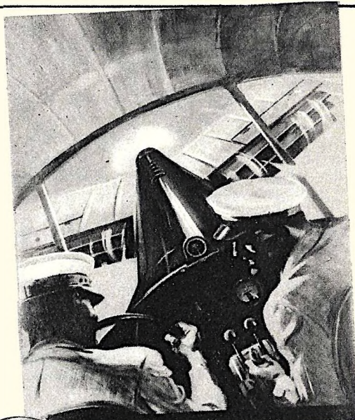
The novel location of the pilot's cockpit affords a striking example of divergence from accepted design. Seated thus at the tail of the plane, the pilot has a commanding view of structure beneath him.
